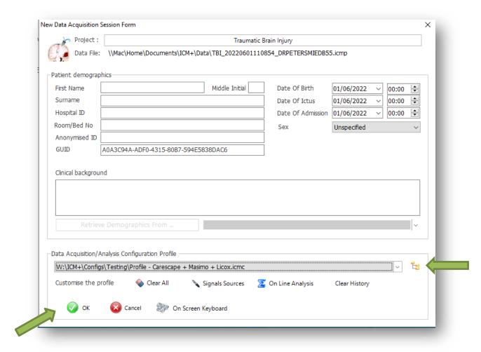
More importantly a data acquisition/analysis profile (configuration) file should be selected, either from the history list box or loaded from the file system. These can then be modified, if necessary, using Signal Sources editor (describe below), and/or On Line Analysis editor.
