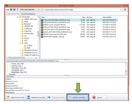
To restore the recording session, the highlighted button must be pressed and the recording resumes using the same profile as when it was closed.
