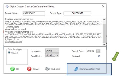
When the connectivity is confirmed the dialog can now be closed, which causes the device to be added to the data collection configuration.
