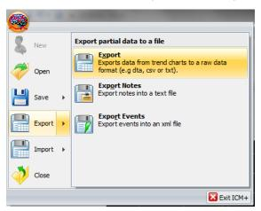
This will export all the trend data from the memory, all the variables, in commas separated columns of values, with the first column containing the time stamps, in the internal Windows DateTime format. The DateTime format is essentially a number of days (and their fraction, which translate into time) since 31/12/1899. Imported into Excel it will initially showed up as those numbers, but if date or time (or combined) cell formatting is requested for that column the data and or time will be shown.
