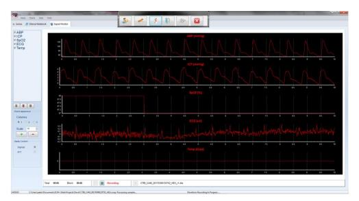
The raw signal monitor, showing all the data as it comes in. Please note that the raw data is stored in a separate file (or files if the one grows too large) with the name shown at the bottom of the monitor signals panel (file extension \*.dta).
