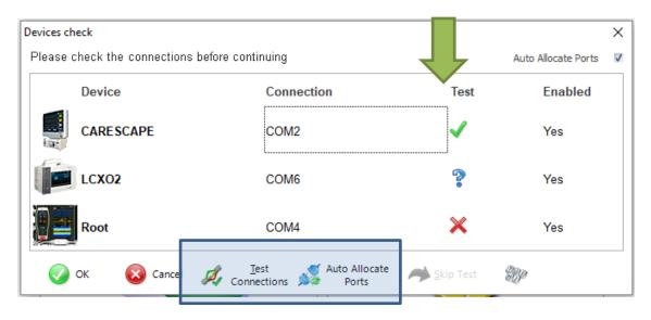
This dialogue is used to test the communication between the ICM+ and the monitor (the 'Test connections' button) and it is also accessible from the Data manu tab later.
