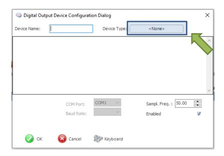
Clicking on the Device type button a list of available, installed, monitor modules will be available to choose from:
