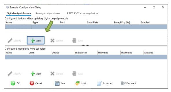
Clicking on Add button in the upper part (Digital Output devices tab) opens a Device Configuration dialog.
