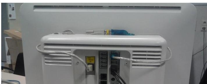
**MX800:** Cable shown connecting the MIB/RS232 port on the Intellivue monitor and the internal PC USB port, using a USB-Serial adapter.
