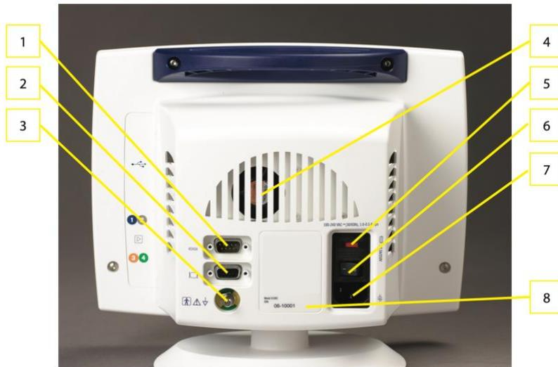
Figure 5-1 Back Connections and Elements
