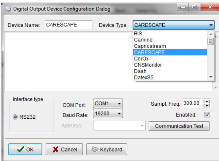
When the correct interface module, the COM port and the baud rate is chosen, clicking on 'Communication Test' will try to establish communication with the monitor and the log of that communication is printed in the memo box, listing also all the parameters that are available to download from the monitor .
