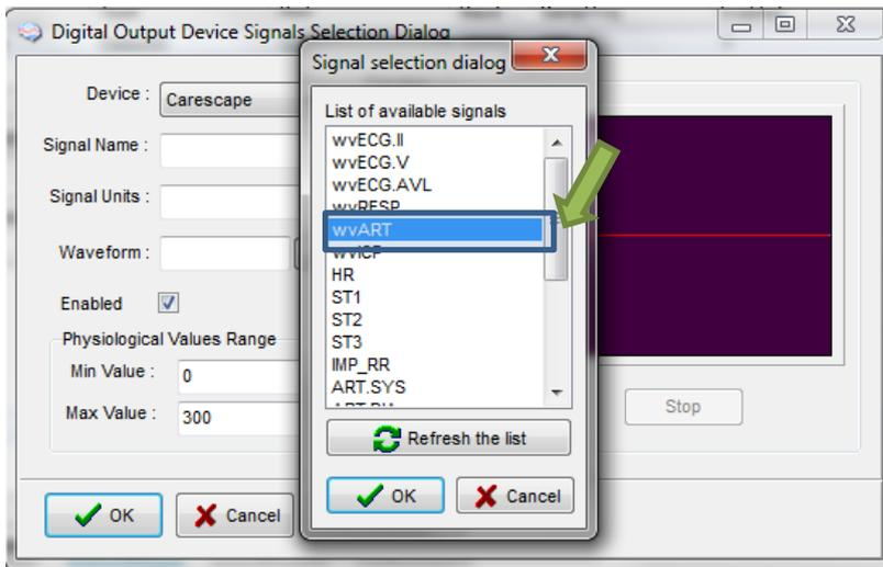
When a parameter is selected one can test if the data is coming in as expected by using the Start button
