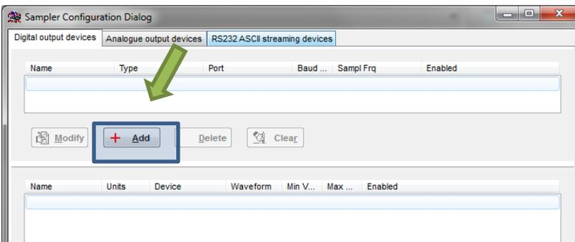
Clicking on Add button in the upper part (Digital Output devices tab) opens a Device Configuration dialog. Here, one can select the monitor module from the list of available (installed) interfaces, as well as specify the serial port (real or virtual, when using USB-RS232 adapter) and its baud rate to match the one configured/offered by the device.
