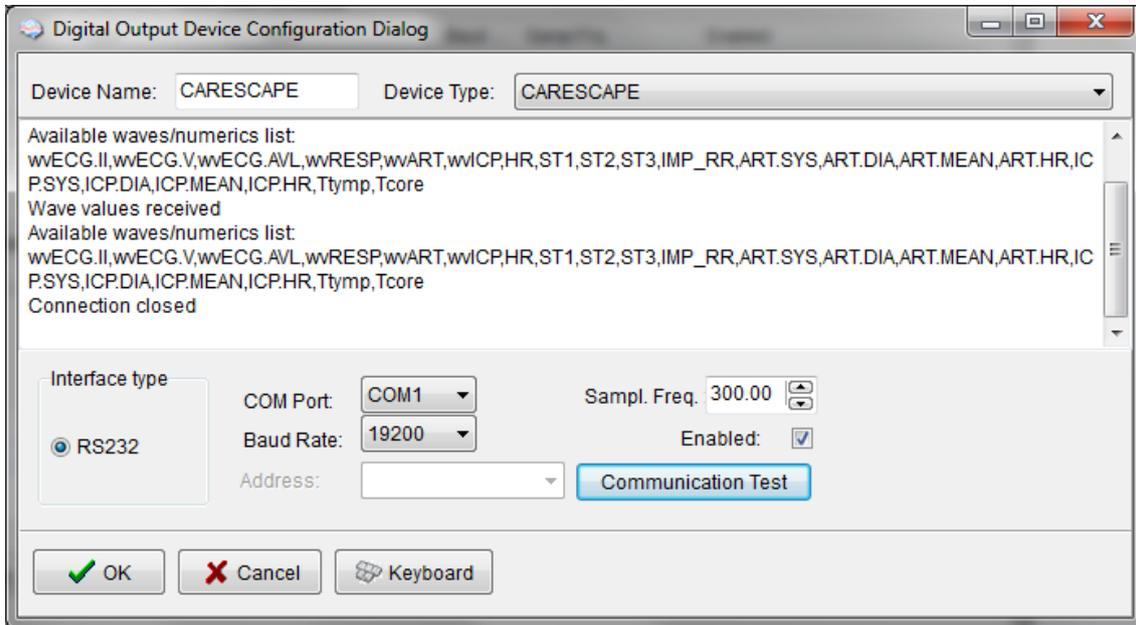
When the connectivity is confirmed the dialog can now be closed, which causes the device to be added to the data collection configuration. What remains to complete the configuration is adding to the configuration all the desired parameters to be downloaded. This can be achieved by using the Add button in the lower part of the Sampler Configuration dialog.
