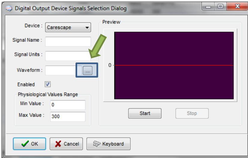
Using the little '...' button one can select available signal, one at a time.
