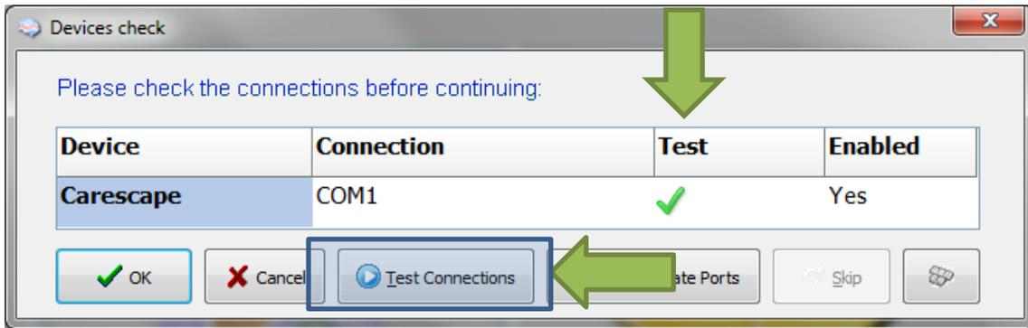
This dialogue is used to test the communication between the ICM+ and the monitor (the 'Test connections' button). If the test is successful the OK button can be pressed.
